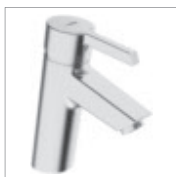
HANSAPINTO XL one-hole single-lever basin mixer, DN 15 4502 2203 chrome without pop-up waste, connection with flexible hoses G 3/8 projection: 102 mm
