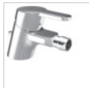
HANSA PRADO one-hole single-lever mixer, DN 15 for bidet 0143 3273 chrome pop-up waste (metal), connection with flexible hoses G 3/8 projection: 125 mm
