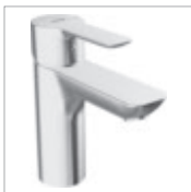
HANSALIGNA one-hole single-lever basin mixer, DN 15 0613 1103 chrome for open hot water heaters, pop-up waste (metal), connection using copper pipes projection: 108 mm
