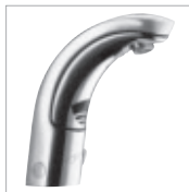
HANSACOBRA electronic basin mixer, DN 15 mains supply 0941 2100 chrome sensory operation (infrared), without pop-up waste, flexible hoses projection: 122 mm
