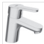
HANSAPRIMO one-hole single-lever basin mixer, DN 15 4942 2203 chrome without pop-up waste, connection with flexible hoses G 3/8 projection: 107 mm
