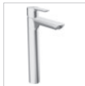
HANSALIGNA one-hole single-lever basin mixer, DN 15 0603 2203 chrome for washbowls, connection with flexible hoses G 3/8, without pop-up waste projection: 150 mm
