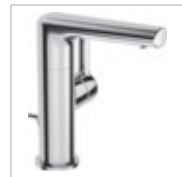
HANSARONDA one-hole single-lever basin mixer, DN 15 5526 2203 chrome spout: swivel, pop-up waste (metal), connection with flexible hoses G 3/8 projection: 115 mm
