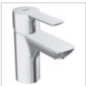
HANSALIGNA one-hole single-lever basin mixer XS, DN 15 0607 2203 chrome pop-up waste (metal), connection with flexible hoses G 3/8 projection: 94 mm
