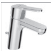
HANSAPRIMO XL one-hole single-lever basin mixer, DN 15 4956 2203 chrome pop-up waste (metal), connection with flexible hoses G 3/8 projection: 110 mm
